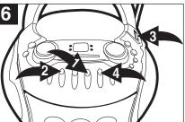
If you wish to listen to your recording immediately, press the cassette REWIND (►►) button • until the tape rewinds to the beginning, then press the STOP/EJECT (■) button • Slide the Function switch • to the TAPE/POWER OFF position, then press the PLAY (◄) button • to begin playback.
